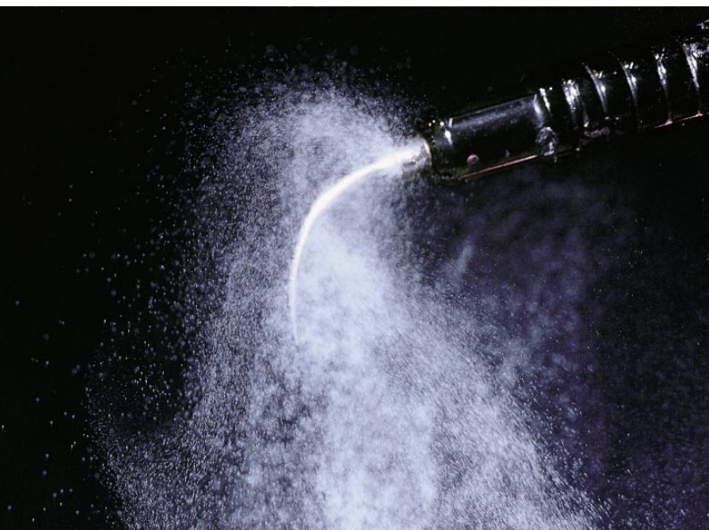
Figure 1. The visible aerosol cloud produced by an ultrasonic scaler using a flow of 17 milliliters per minute of coolant water.
